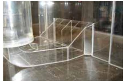
Model of a Flygt FSI used in the tests.
