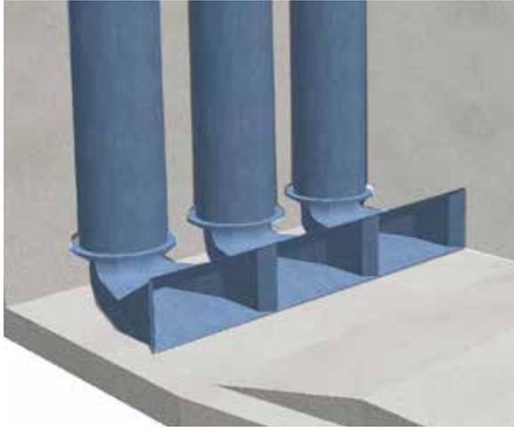
An alternative to a formed suction intake design is the Flygt Formed Suction Intake (FSI), a specially engineered device for propeller pump intakes. With the Flygt FSI, it is possible to design an even more compact station. Compared to the already compact Flygt standard open sump intake design, the Flygt FSI helps reduce the footprint of the sump by up to 60%. The Flygt FSI is capable of normalizing even higher flows than those handled by a formed suction intake design.
