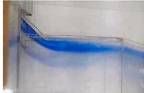
The difference in flow without chamfers and with chamfers.
