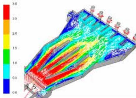
CFD simulation of modified design.
