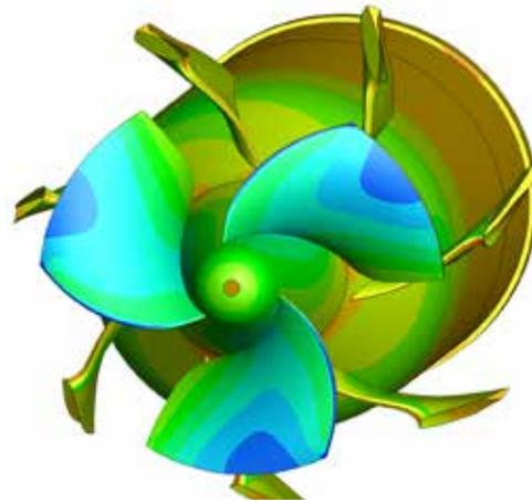
CFD model of a complete pump with a rotating propeller (pump housing removed for clarity); colors indicate pressure on the blades and other internal surfaces.
