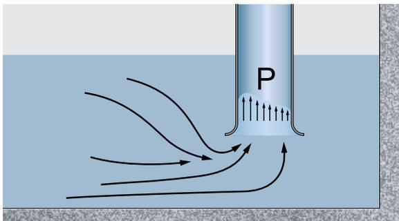
Uneven velocity into the pump inlet.
