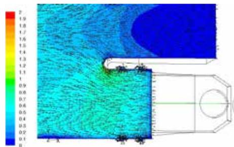
CFD simulation of modified design with uniform flow.
