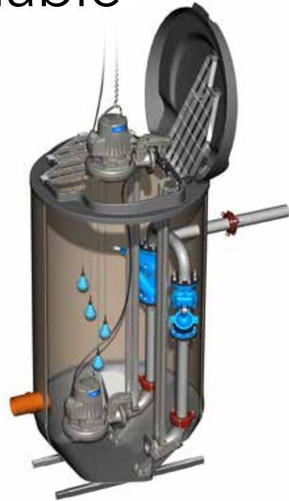
In a two-pump station, four level regulators are generally used. One is positioned at the stop level, one at each pump's start level, and the fourth regulator is used to trigger a high level alarm.
