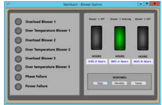
Blower station status screen
