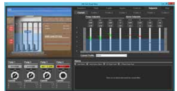
Lift Station number status screen
