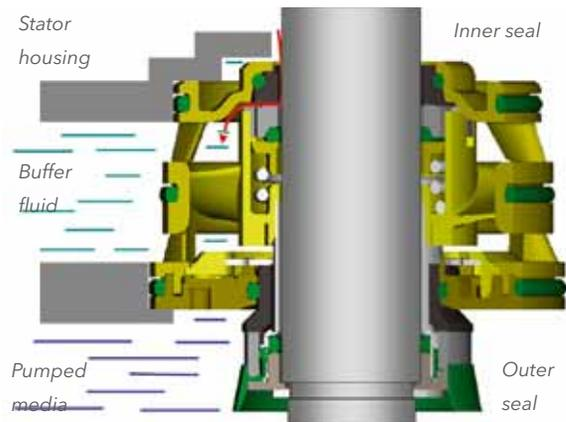
Active Seal applied in a Flygt Plug-In Seal. Any buffer fluid that may leak into the stator housing is immediately pumped back to the buffer fluid chamber.
