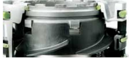
*The cooling pump propeller.*
