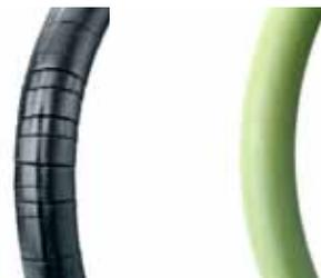
*O-rings in nitrile (left) and viton after testing at 392°F.*
