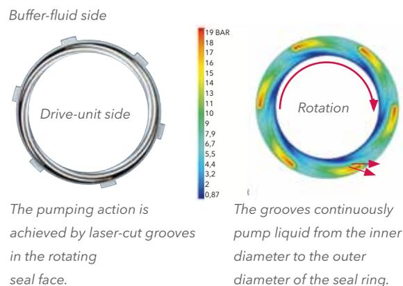
The pumping action is achieved by laser-cut grooves in the rotating seal face.
