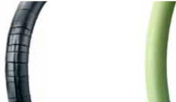
O-rings in nitrile (left) and viton after test at 392°F.
