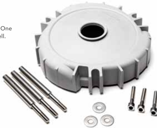
Diffusor kit including diffusor, hexagon head screws, plain washers, barrel nuts and a mounting instruction.
