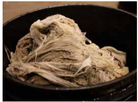
Debris pulled from a lift station.
